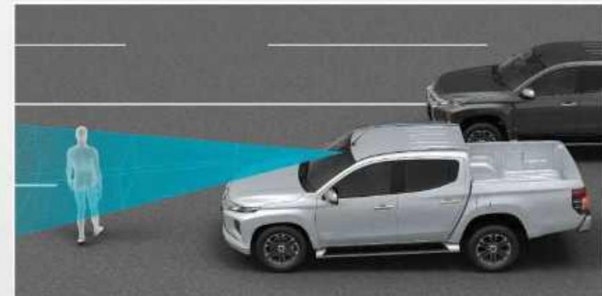
**Forward Collision Mitigation System [FCM]<sup>6</sup>**
